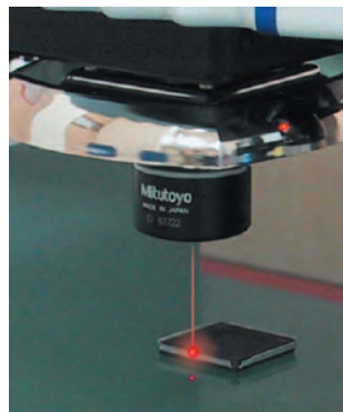
Coaxiale laser Tracking Auto Focus (TAF)
