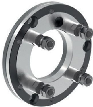
A09 Steel Intermediate flange according to DIN ISO 702-3 (DIN 55027) / cylindrical mount on chuck side according to DIN 6350
