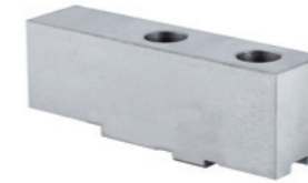
A09 Top jaw AB, special length, soft, material 16MnCr5, DIN 6350
