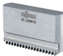
A28 Unstepped jaw BL, 3-jaw set diagonally toothing, unstepped, soft, material 16MnCr5
