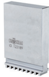
A09 Unstepped jaw BL, special height, soft, material 16MnCr5, DIN 6350
