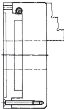
ZS Hi-Tru, with one set outward stepped jaws and one set inward stepped jaws, DIN 6350, cylindrical centre mount, form A
