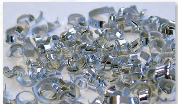
With 3D-chip breaker: Breakage chips
