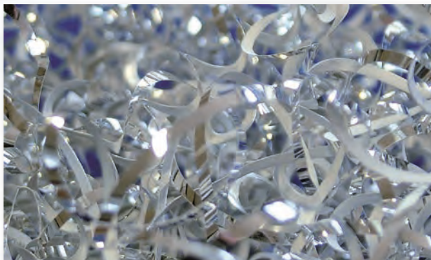
Without 3D-chip breaker: Flow chips
