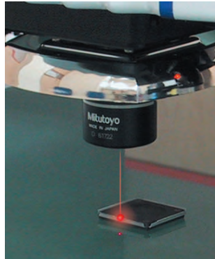
Coaxiale laser Tracking Auto Focus (TAF)
